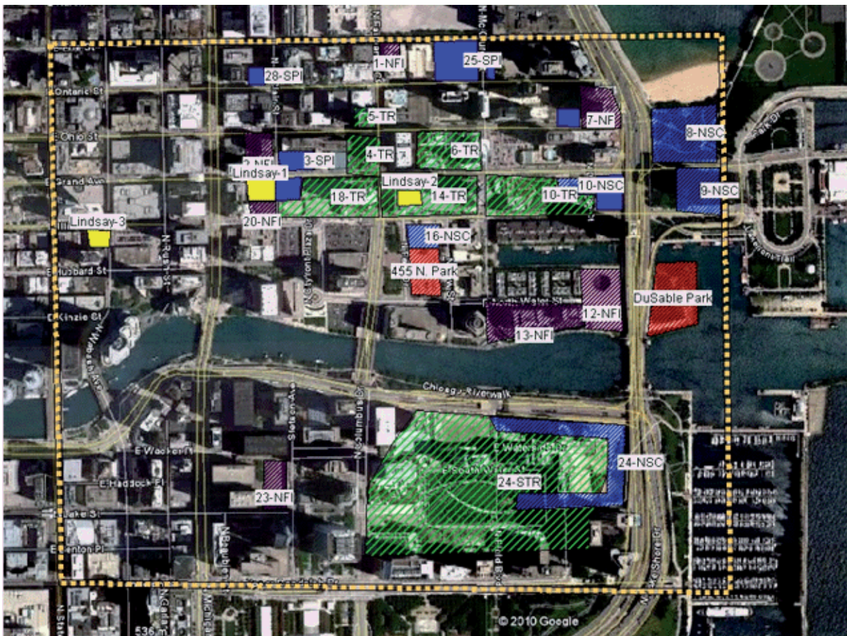
Screen dump from GeoMap displays a survey area with different types of contaminated and remediated sites.
